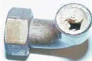
**Photograph 8. Brass fitting affected by meringue dezincification**
