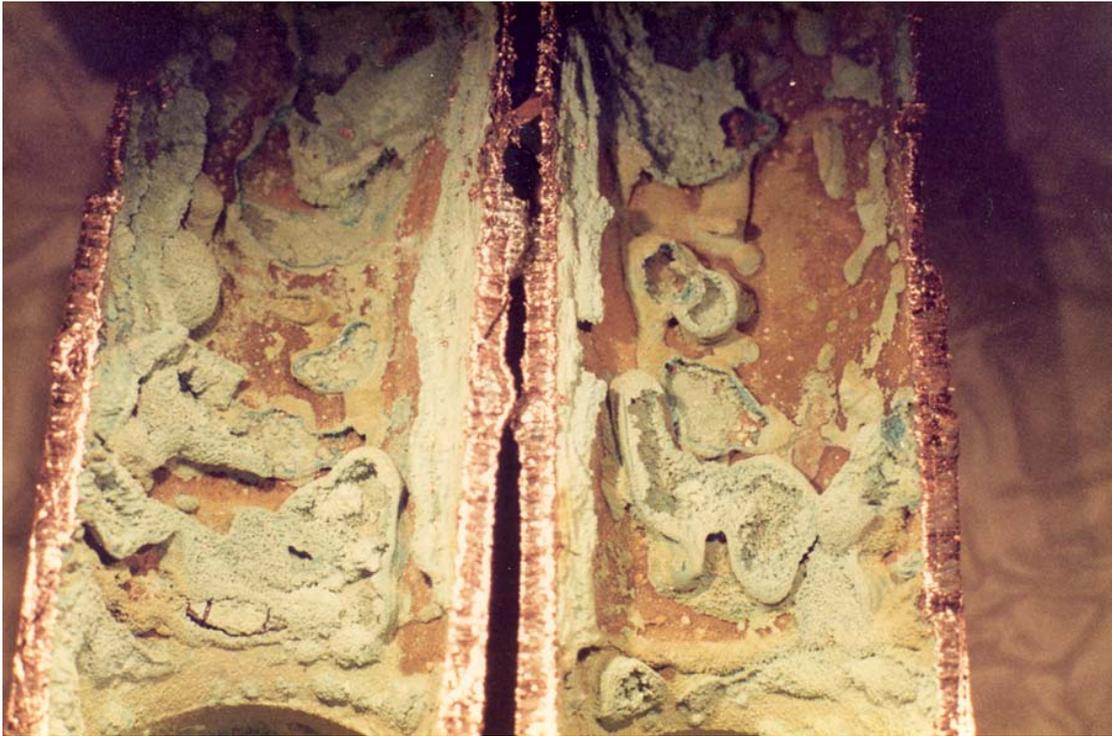
**Photograph 5. Voluminous corrosion deposits produced by soft water**
