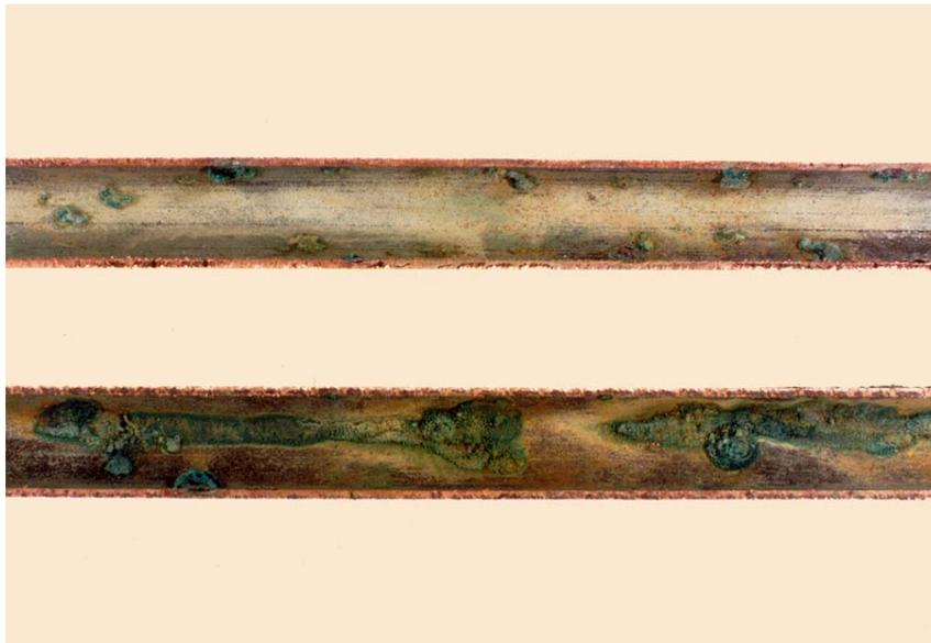
**Photograph 3. Typical distribution of Type I pits in copper pipe**
