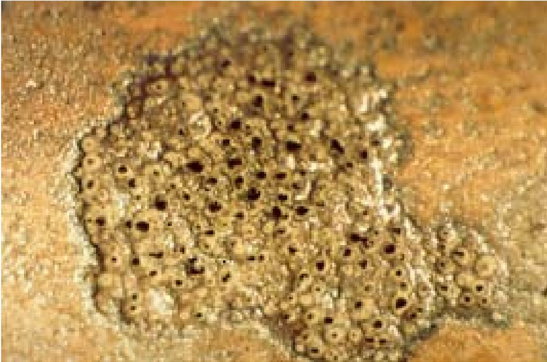
**Photograph 7. An acid cleaned copper pipe surface showing ‘pepper pot corrosion’ produced by microbiological action**
