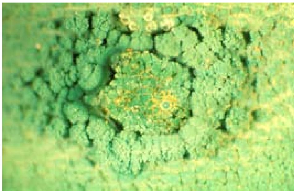
**Photograph 4. Detail of a Type I pit with a central mound of malachite above the initiating site surrounded by secondary mounds above daughter pits**
